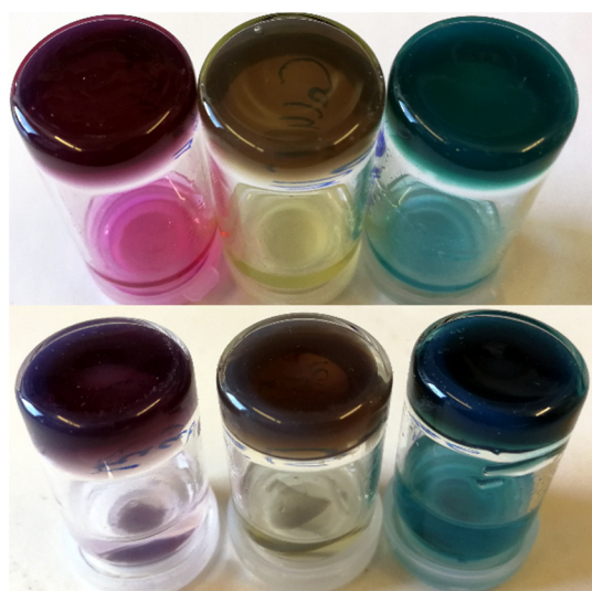
Figure 11. Metallogels with dye solutions as prepared and used for UV experiments. The upturned vessels shows the retained gel state of the samples. Top: Dye uptake after 7 days.
